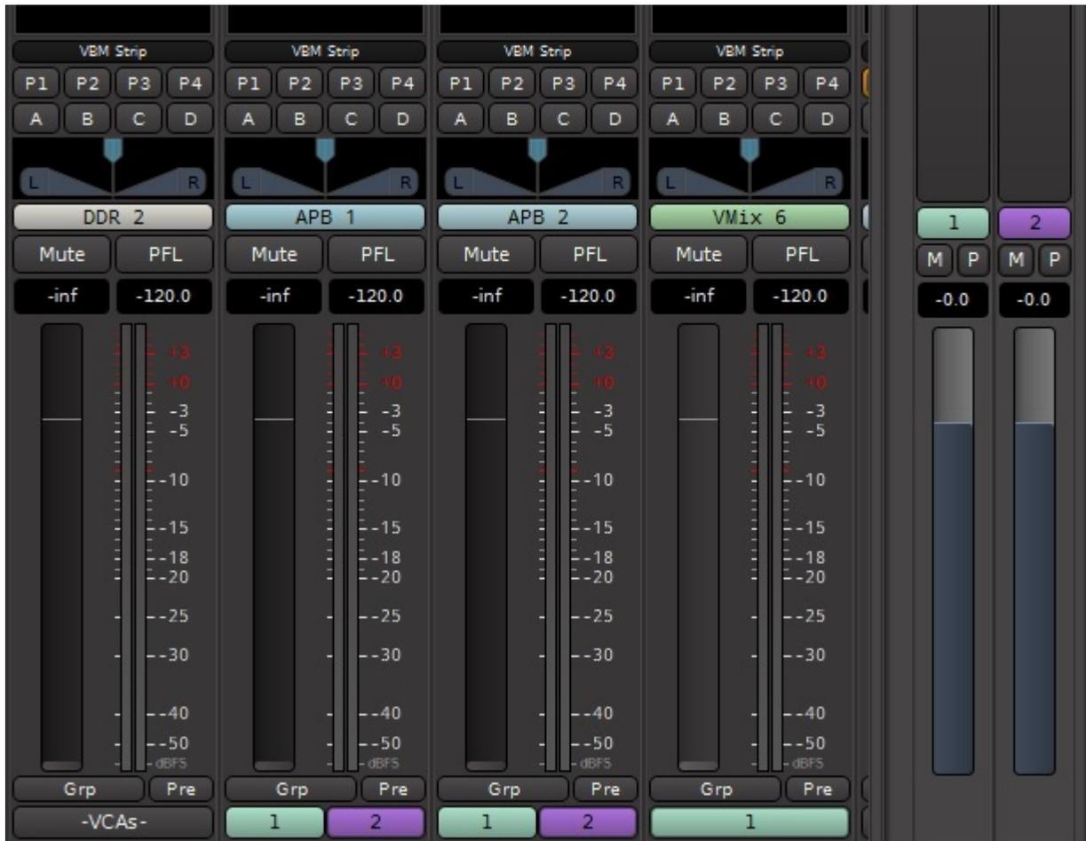
Clicking on the VCA assign button will allow additions or changes to VCA assignments, as shown in [Figure 23](#). VCA assignments or deassignments are made by clicking in the checkboxes. The "Unassign All" option simultaneously disconnects the channel or bus master from all VCA masters it is assigned to, and does not appear when the channel is not assigned to any VCA master.
