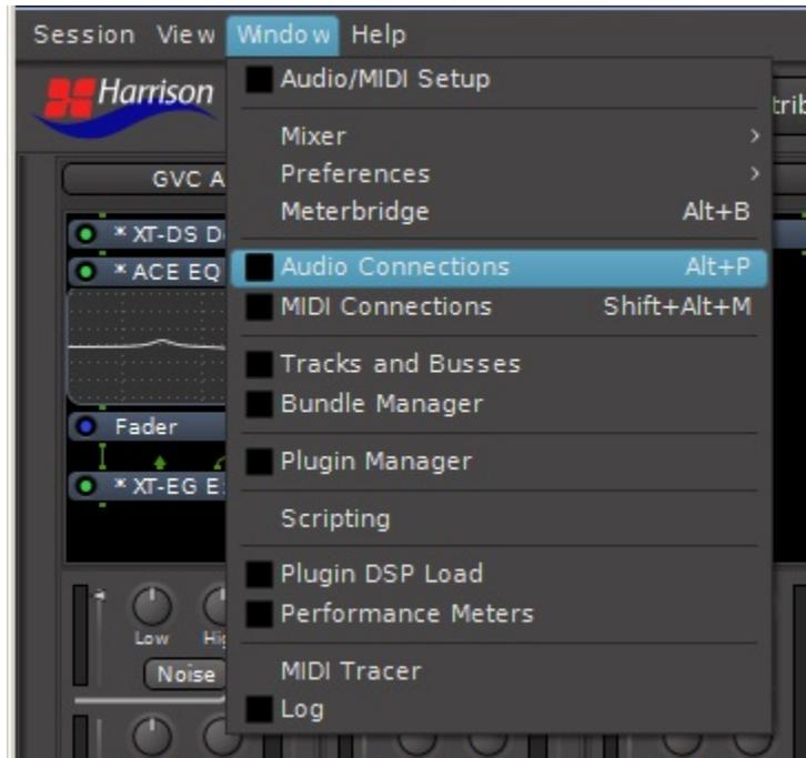
One example of the Routing Tool is shown in [Figure 44](#). With the Routing tool any desired audio connections may be made. It is used particularly for connecting Channel inputs and Bus outputs to physical I/O hardware (or network I/O) .
