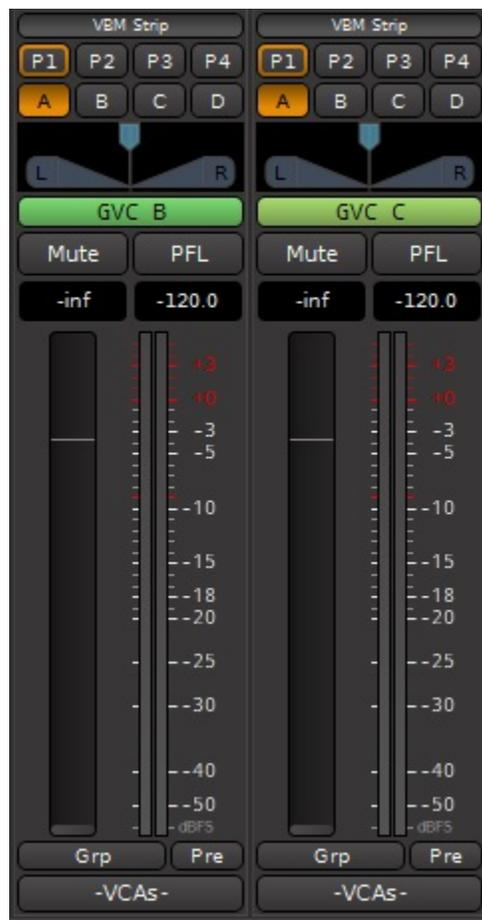
On normal (non-contributor) input channels Lobby selections operate as an additional program bus, signal can be assigned to either program bus or lobby, or both. When the fader is down, Lobby and program sends are inactive, i.e. both sends are post-fader.
