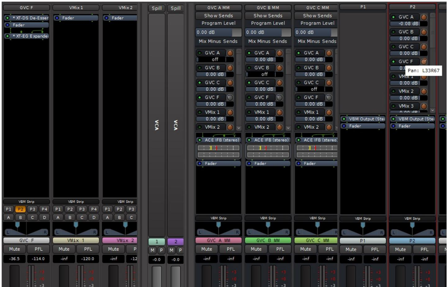
The Sends section provides the capability to customize the mixes on each MixMinus and Program bus. However these are advanced features and must be used with considerable caution otherwise you will end up with an unexpected mix. For example, turning off a send level here will defeat the function of the associated channel fader to ALL of its destinations.
