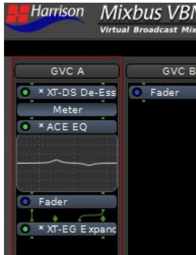
In the figure, the custom metering point is between the first two plugins before the fader. As with any plugin (or the fader itself), its position in the signal flow can be changed simply by dragging it up or down.
